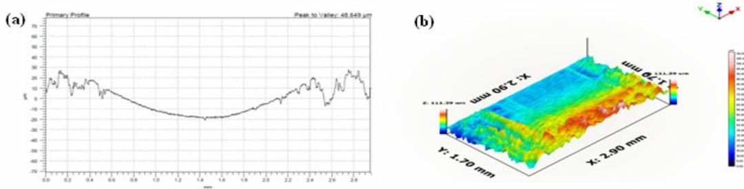
Figure 3. Surface profile of CoNiCrAlY coatings produced by APS wear tested against (a) substrate, and (b) surface topography of the worn coating
