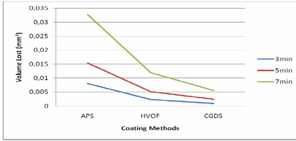
Figure 1. Volume losses as a result of erosion according to coating method
