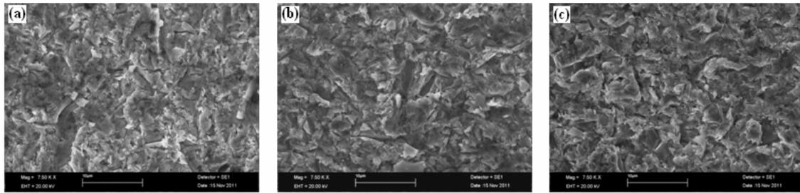
Figure 5. SEM micrograph of the wear track on the CoNiCrAlY coatings; (a) APS- CoNiCrAlY coatings, (b) HVOF- CoNiCrAlY coatings, (c) CGDS- CoNiCrAlY coatings
