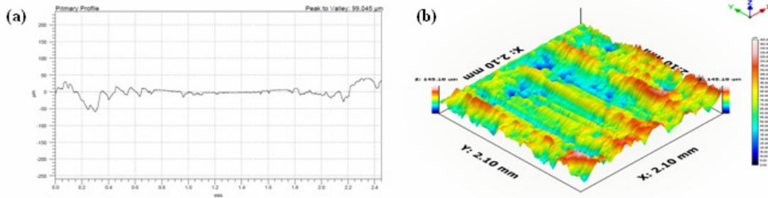
Figure 2. Surface profile of CoNiCrAlY coatings produced by CGDS wear tested against (a) substrate, and (b) surface topography of the worn coating
