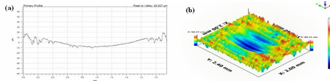
Figure 4. Surface profile of CoNiCrAlY coatings produced by HVOF wear tested against (a) substrate, and (b) surface topography of the worn coating
